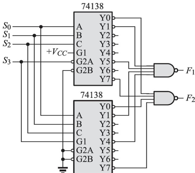
(A)  $F_1(S_3, S_2, S_1, S_0) = (1, 5, 9, 12)$  且  $F_2(S_3, S_2, S_1, S_0) = (0, 7, 8, 15)$  (B)  $F_1(S_3, S_2, S_1, S_0) = (0, 7, 8, 15)$  且  $F_2(S_3, S_2, S_1, S_0) = (1, 5, 9, 12)$  (C)  $F_1(S_3, S_2, S_1, S_0) = (1, 5, 8, 11)$  且  $F_2(S_3, S_2, S_1, S_0) = (0, 7, 8, 14)$  (D)  $F_1(S_3, S_2, S_1, S_0) = (2, 3, 4, 6)$  且  $F_2(S_3, S_2, S_1, S_0) = (2, 3, 4, 6)$
